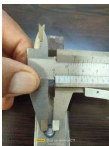
Figure 2: resistance spot Welding measurement.
