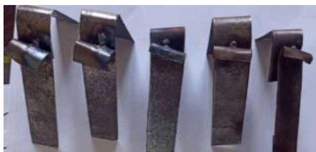
Figure 4: Peel test for spot TIG welding.
