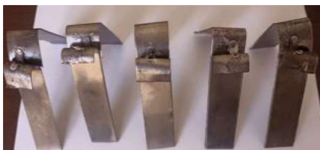
Figure 5: peel test for resistance spot welding.
