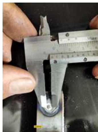
Figure 3: TIG Spot Welding measurement .
